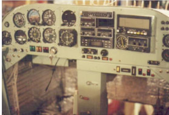
**The finished instrument panel, already installed and tested.**
