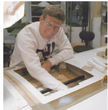
**The control stick grows out of linkage buried in the wings.**
