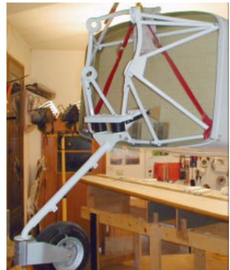
**The Glassair Super II FT engine mount and nose gear.**
