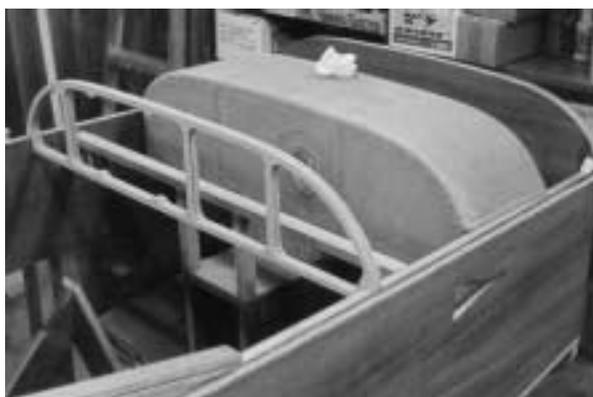
**Instrument Panel, Header Tank, and Firewall.**
