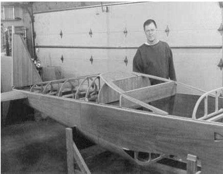
**Mike Rieff and the GP-4 fuselage. The notch under the cockpit will sit over the wing. The near-horizontal hoop surrounding the cockpit is the base for the sliding canopy frame.**
