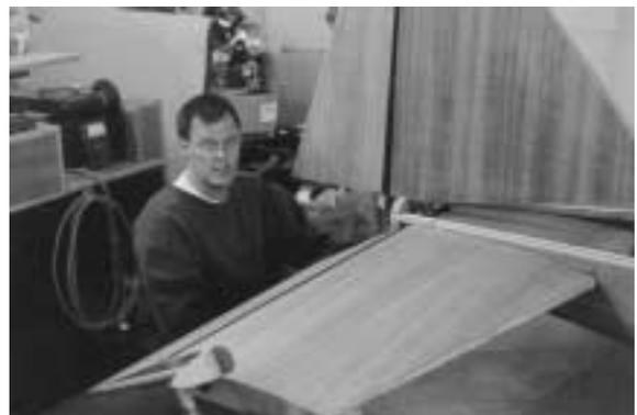
**“The tail-cone is fiberglass, attaches to the bulk-head here, and fairs the rudder and elevators into a point.”**
